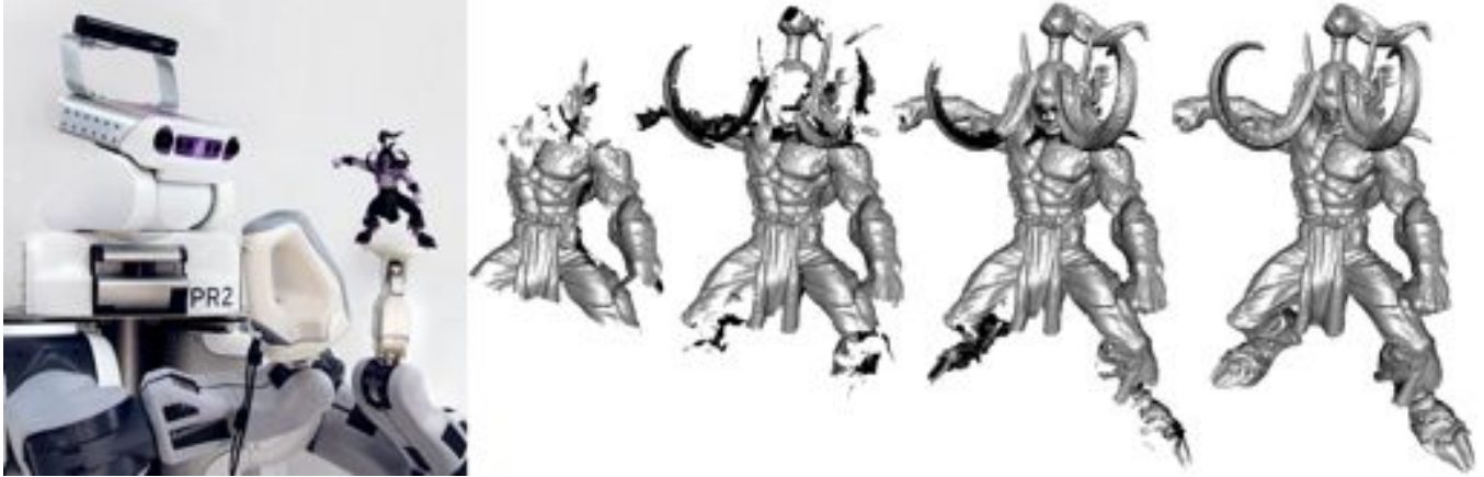
Figure 1: Our robot-based, Poisson-guided autoscanner can progressively, adaptively, and fully automatically generate complete, high quality, and high fidelity scan models.
