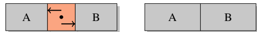
Figure 2: Overlap removal in Box2D: Solving body-to-body constraints by pushing bodies away from each other with applied forces.
