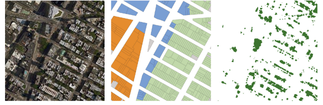
Fig. 3. Urban layout: satellite images (left), zone data for individual lots (middle), and coverage maps (right) are available in public datasets. We use zone data and lot geometry as inputs to our procedural models and learn to predict their parameter values from the coverage maps.
