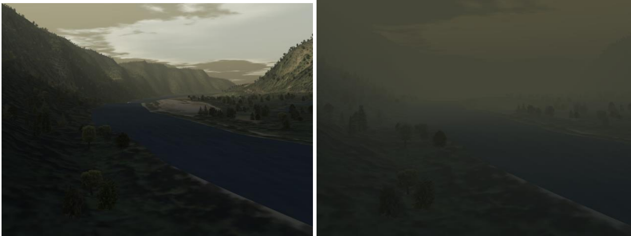
Figure 4. Simulated cockpit view of identical point with varying visibility conditions (12 km on the left, 1200 m on the right), seen at a height above ground of 80 ft.
