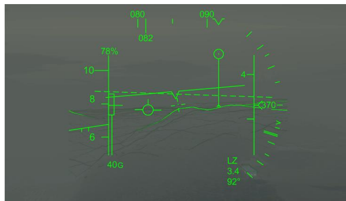
Figure 9. 3D conformal symbology (terrain grid with contour lines) overlaid with 2D symbology supplemented with a display of the waypoint denoting the landing zone.
