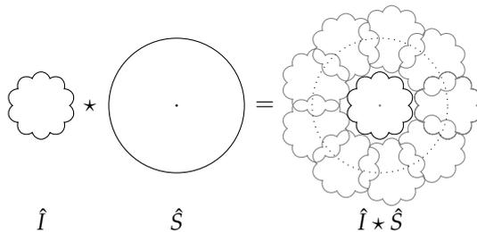
Figure 3: The spectrum of the sampled signal  $\hat{I}_s$  is obtained by convolving the original spectrum with the Fourier transform of the sampling function. Aliasing occurs when the replicated spectra  $\hat{I}$  overlap the central spectrum on the right-hand side.
