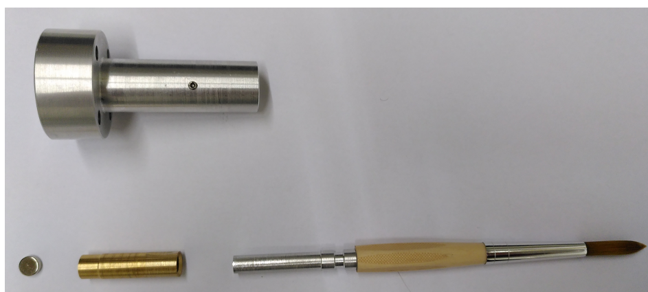
(c) The individual components of the brushholder, from left to right and top to bottom: Holding tube, magnet, brass sleeve, adapter with brush.
