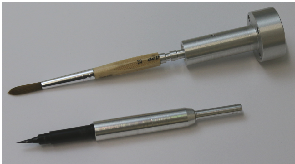
(b) The new brushholder with a tool adapter
