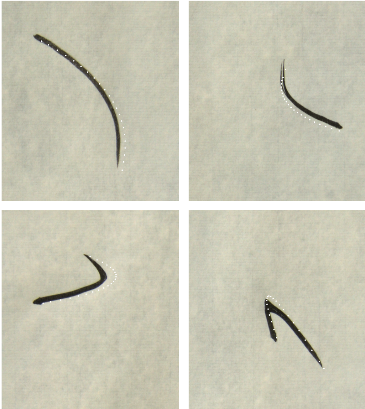
Figure 6. Strokes collected during a run of the recording system. Each rectangle is 10 cm × 10 cm and the strokes have been generated from random cubic Bézier curves. The white dots indicate the robot tool center point (TCP) path along the canvas and the deviation induced by brush lag is visible.
